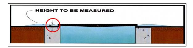
Example: The measured height of the plume exiting the ring of a 36-inch manhole is 1 inch. The total volume per minute would be 13 gpm from around the ring of a 36-inch manhole cover (from the attached chart). (Calculate the amount exiting the pick hole(s) and add to the total being lost around the ring). If the SSO lasted one hour the total wastewater lost would be 780 gallons ( $13 \times 60 = 780$ ).
