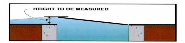
Example: The measured height of the plume exiting the side ring of a 24-inch manhole is 2 inches. Based upon the data provided in the Area Calculation Chart below, a 2-inch plume from one side of a 24-inch manhole cover provides 0.524 square feet of area. The velocity of the flow is estimated at 4 ft/sec (visual observation) with the assumed duration of the flow lasting for one hour. The total amount of the SSO is estimated at 56,441 gallons ( $.524 \times 4 \times 60 \times 7.48 = 56,441$ )
