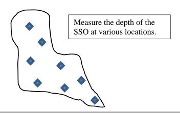
Where it is difficult to measure wet spots on asphalt, use a depth of 0.0026' or 1/32". For wet spots on concrete use depths of 0.0013' or 1/64" for reasonable estimates.
